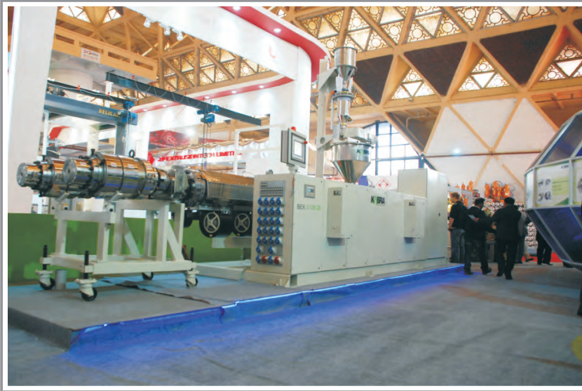
Twin Screw Extrusion Line (PVC Pipe)
