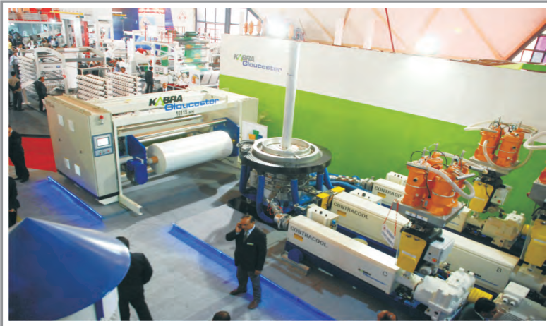
Extruders, Die Header Winder, KAGE 3-Layers Blown Film Plant
