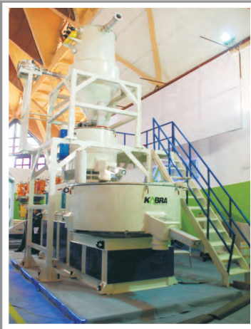
High Speed PVC Compounding Mixer Cooler
