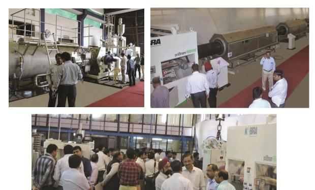
The demonstrated plant comes with special features like – next generation grooved feed design, servo haul off, swarfless pipe cutting, gravimetric system for weight/meter control, and output of 1200 Kg/hour. The larger processing window of 40:1 L/D, helps in obtaining excellent linear specific output even for heavier grade material - higher than PE 100.
